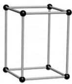
Tetragonal a = b \neq c \alpha = \beta = \gamma = 90^\circ
