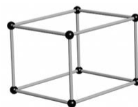
Monoclinic a \neq b \neq c \alpha = \beta = 90^\circ, \gamma \neq 90^\circ
