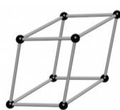
Rhombohedral a = b = c \alpha = \beta = \gamma \neq 90^\circ
