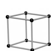
Cubic a = b = c \alpha = \beta = \gamma = 90^\circ
