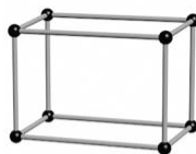
Orthorhombic a \neq b \neq c \alpha = \beta = \gamma = 90^\circ
